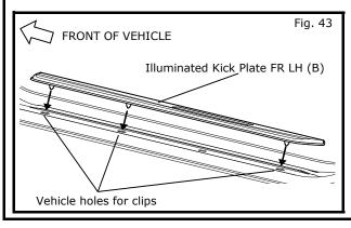
29) Align Location Clips (E) on Illuminated Kick Plate FR LH (B) to vehicle holes (first, second & fourth) as shown in Fig.43.
