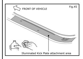
32) Clean the Illuminated Kick Plate attachment area as shown in Fig.45 with 50/50 alcohol/ water, let dry for 30 seconds.
