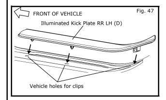
34) Align Location Clips on part to first and second holes on vehicle from front side as shown in Fig.47.
