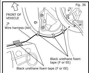
22) Route wire harness (AA) along vehicle parking brake cable as shown in Fig.36.
