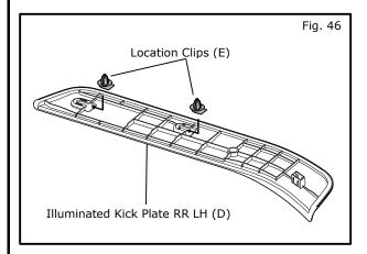
33) Slide Location Clip (E) into the clip seat of backside of Illuminated Kick Plate RR LH (D) as shown in Fig.46.
