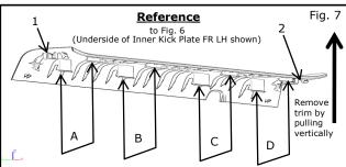
Important: Clips are located at locations labeled; 1, 2, and A thru D in Fig.6 and Fig.7. Note locations and orientations to avoid damage.
