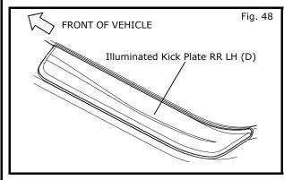
35) Insert Location Clips to vehicle hole and push down to lock clips as shown in Fig.48.
