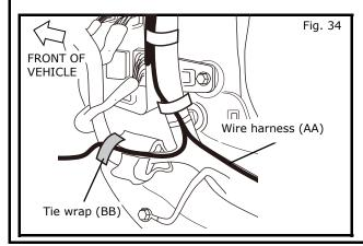
20) Route wire harness (AA) and secure to vehicle harness by tie wrap (BB) as shown Fig.34. (1 place)
