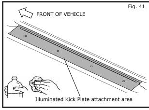
26) Clean the Illuminated Kick Plate attachment area as shown in Fig.41 with 50/50 alcohol/ water, let dry for 30 seconds.
