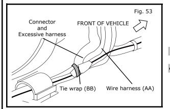
40) Secure the connector of wire harness (AA) and excessive harness to vehicle harness with tie wrap (BB) as shown in Fig.53.
