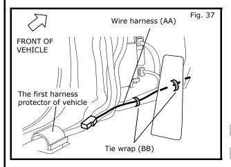
23) Route wire harness (AA) along vehicle harness and the connector of wire harness (AA) in front of the first harness protector of vehicle as shown in Fig.37.
