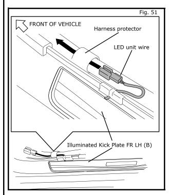
38) Route LED unit wire of Illuminated Kick Plate FR LH (B) into harness protector as shown in Fig.51.
