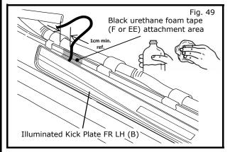
36) Clean both sides of the attachment area for the black urethane foam tape (F or EE) with 50/50 alcohol & water, let dry for 30 seconds as shown in Fig.49.
