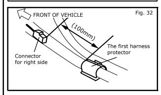
17) Align the connector for right side at about 100mm in front of the first harness protector of vehicle as shown in Fig.32.
