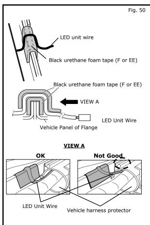
37) Place black urethane foam tape (F or EE) over flange, then place the LED unit wire on top of the black urethane foam tape (F or EE) as shown in Fig.50. Apply second black urethane foam tape (F or EE) on top of the LED unit wire as shown in Fig.50.
