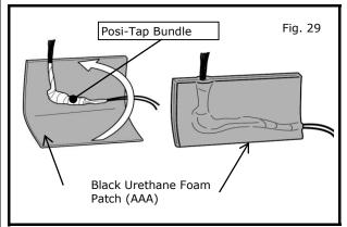
11) Place secured Posi-tap bundle on sticky side of black urethane foam patch (AAA), then fold in half as shown in Fig29.
