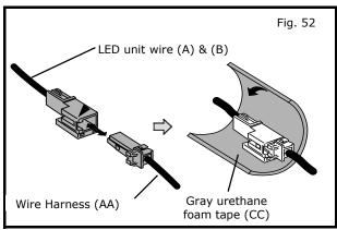
39) Connect LED unit wire (B) to wire harness (AA) then cut one piece of gray urethane foam tape (CC) in half, apply one half around connecting section as shown in Fig.52.
