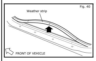
25) Remove the front door weather strip as shown in Fig.40.
